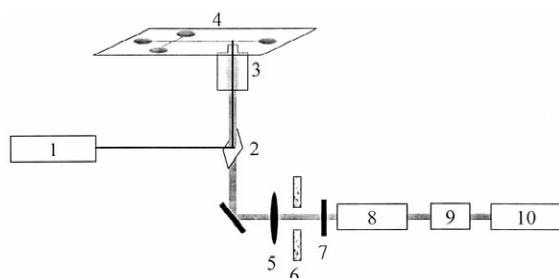
Fig. 2. Block diagram of the laser-induced fluorescent, confocal detection apparatus of the electrophoresis microchip system. (1) NdYAG laser, (2) dichroic mirror, (3) microscope objective, (4) glass electrophoresis microchip, (5) achromatic lens, (6) spatial pinhole filter, (7) band-pass filter, (8) photomultiplier, (9) low-noise preamplifier, (10) data acquisition system.
